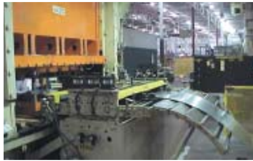
Whirlpool installed a 50-in. light-gauge press feed system with a stock reel and coil car, coil straightener, and four-roll servo feeder on a cabinet stand to solve its press feeding problems with downtime caused by die jams.
