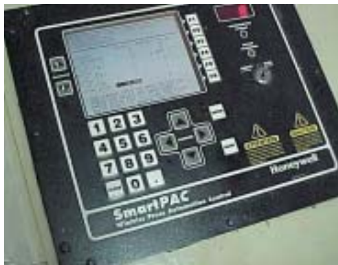
The company also acquired a press interface and control system that features parameters that can be set, in-die sensing, and tonnage monitoring.
